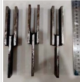
Rubber Shear Modulus Test Specimens
