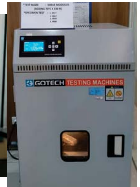
Anaerobic Ageing Conditioning equal to 60 years condition
