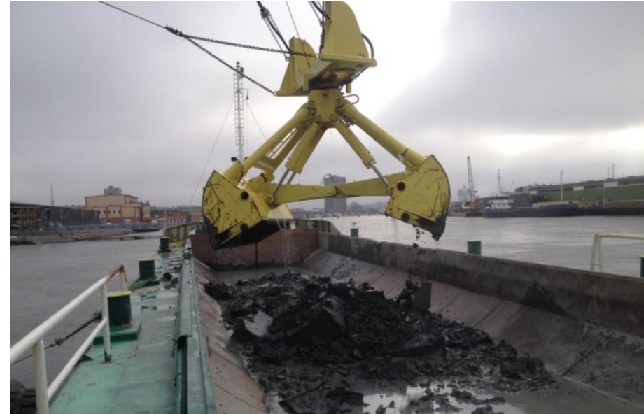
Grab dredger, Kahmari 2 with 16 m 3 Horizontal Profiling Grab + split hopper barge, case study : The Marieholm tunnel in Sweden
