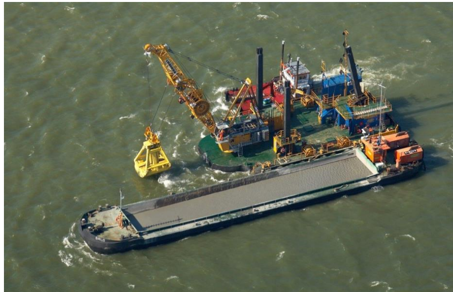
Grab dredger, Kahmari 2 with 16 m 3 Horizontal Profiling Grab + split hopper barge, case study : The Marieholm tunnel in Sweden
