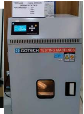
Anaerobic Ageing Conditioning equal to 60 years condition
