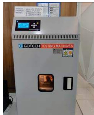
Anaerobic Ageing Conditioning equal to 60 years condition
