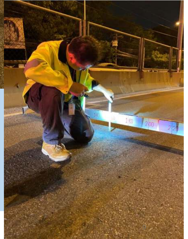
Rut Depth Measurement
