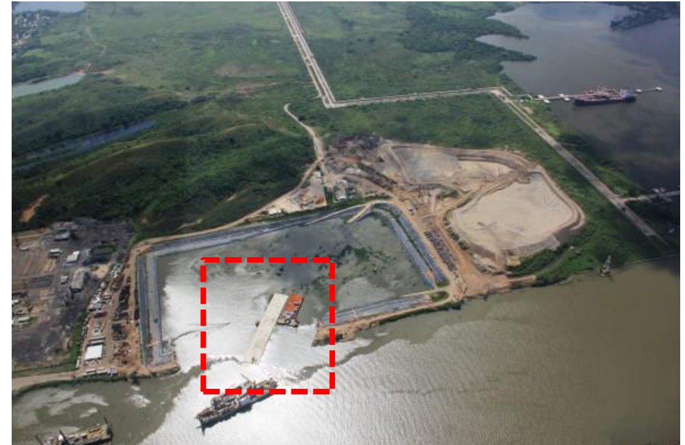
Casting basin just before inundation (left) and casting basin after inundation with one tunnel element floating (right)- case study : The Coatzacoalcos tunnel in Mexico
